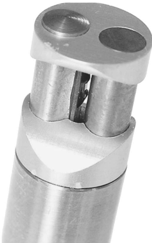
FIG. 2. The commercially available PU probe, with the particle velocity sensor packaged in between the two cylinders.
